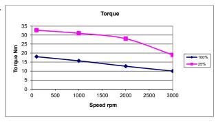
Data were measured on an HDD14N-Pa series motor mounted on a vertical 450 x 375 x 30 mm steel plate in free air, with a winding temperature rise of 90°C and driven by a commercially available inverter.
