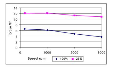
Data• were measured on an HSM 09Q-Pa series motor mounted on a vertical 260 x 200 x 12 mm aluminum plate in free air, with a winding temperature riseof 90°C and driven by a commercially available inverter.
